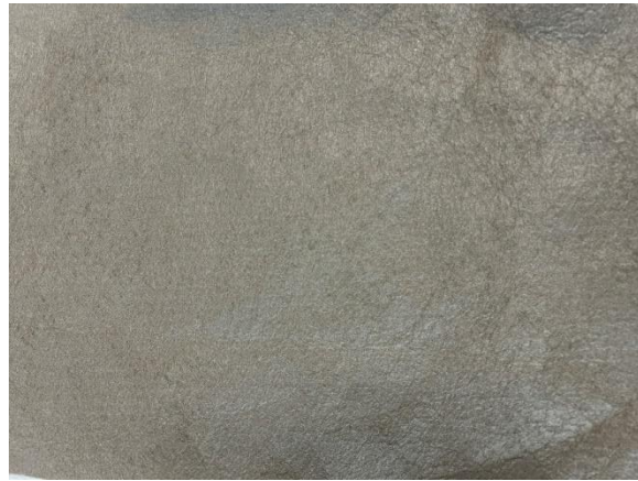
Figure 3. Texture of Nonwoven geotextile
