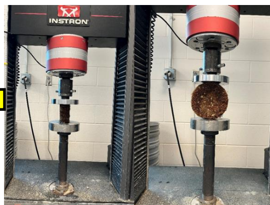
Small-scale and large-scale lab wetting and drying (Durability) tests on fiber-based concrete mixtures
